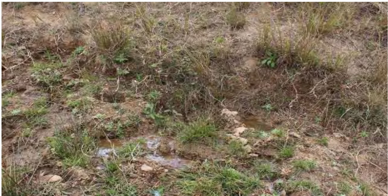
Seepage at the toe and upper right flank
